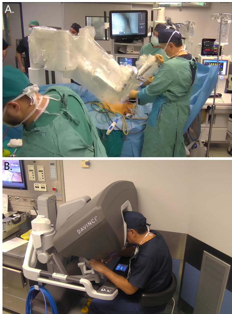
Figure 1. Operating room images of the da Vinci X® robotic surgical system: (A) patient cart positioning and surgical arms docking, (B) surgical console providing control of all four arms and three-dimensional vision of the surgical field.
